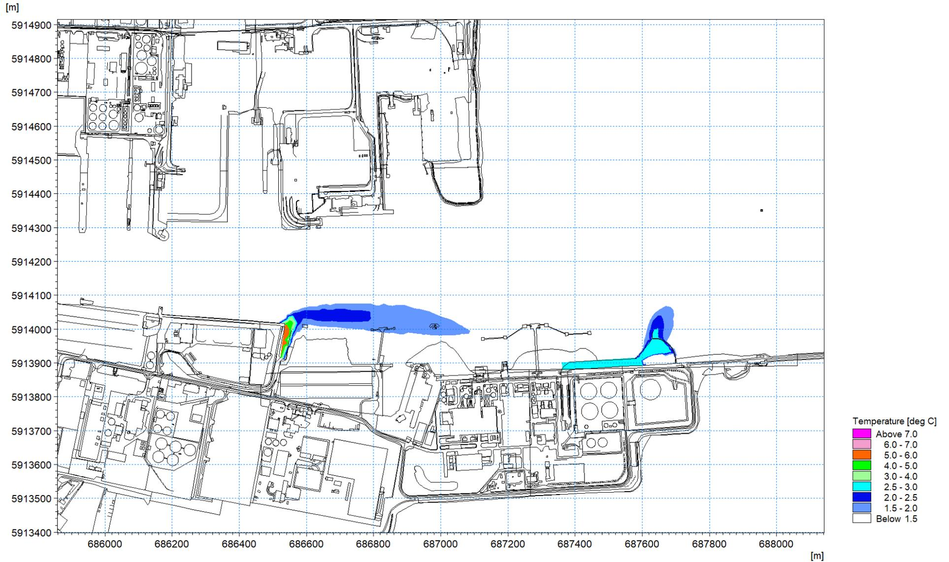
Figure 1.79: Thermal plume 12<sup>th</sup> August 2016 – excess temperature at mid-flood circa 0.3m depth layer 6
