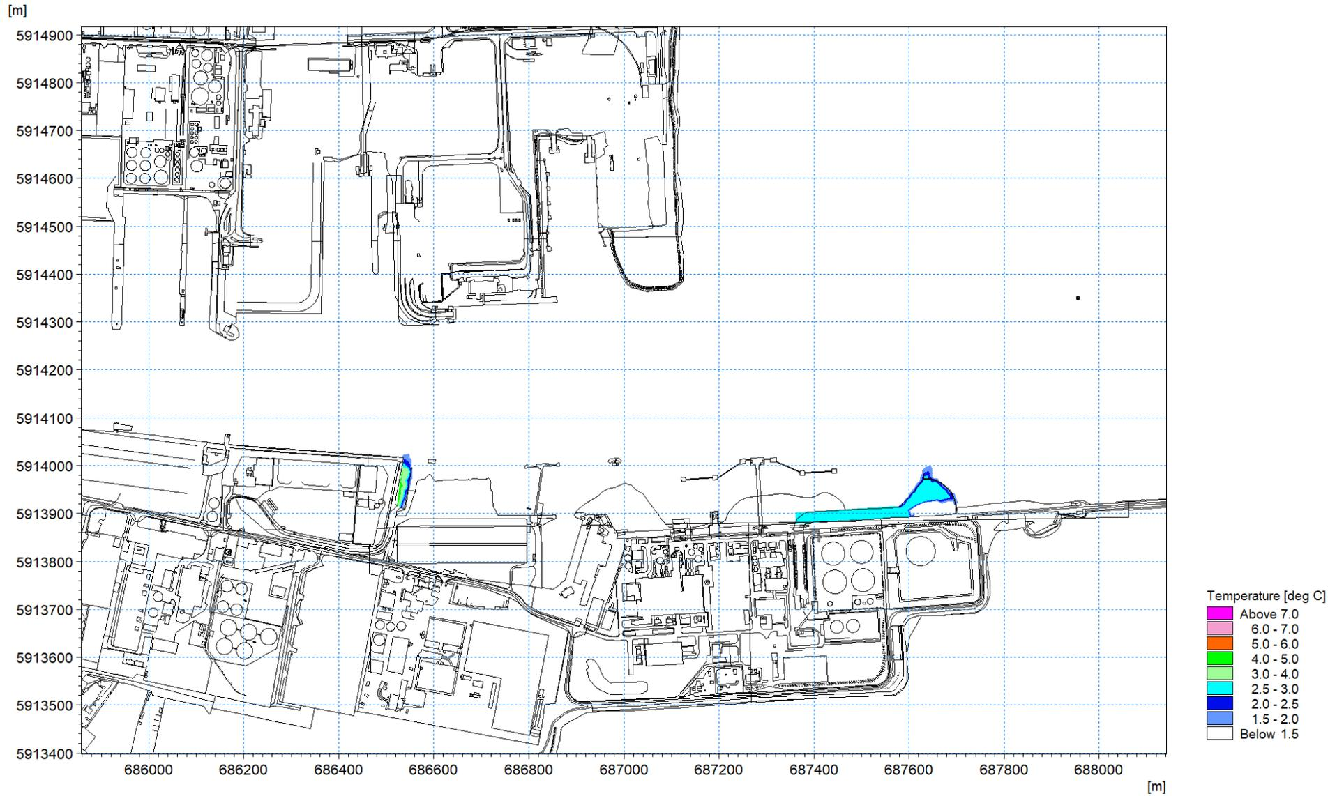
Figure 1.72: Thermal plume 12<sup>th</sup> August 2016 – excess temperature at high water circa 2m depth layer 4
