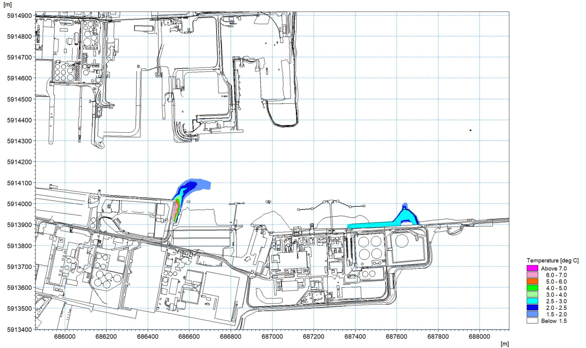
Figure 1.98: Thermal plume 24<sup>th</sup> April 2018 – excess temperature at high water circa 1m depth layer 5
