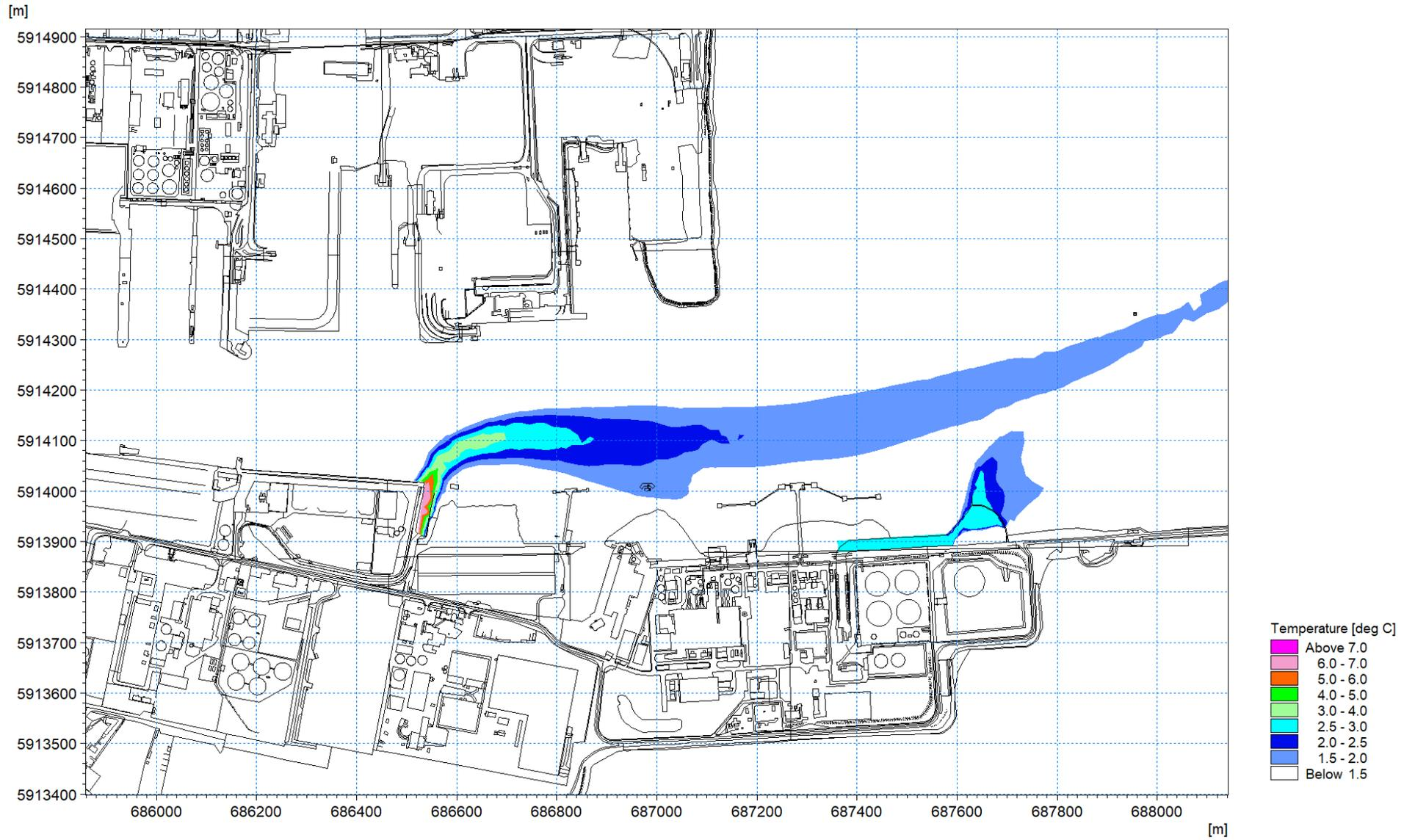
Figure 1.100: Thermal plume 24<sup>th</sup> April 2018 – excess temperature at mid-ebb circa 0.3m depth layer 6
