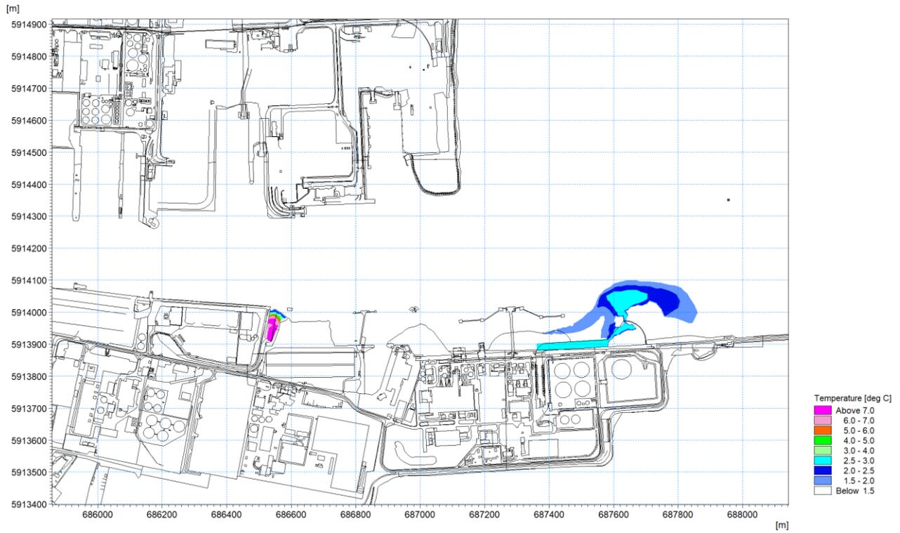
Figure 1.31: Thermal plume 20<sup>th</sup> April 2018 – excess temperature at low water circa 0.3m depth.
