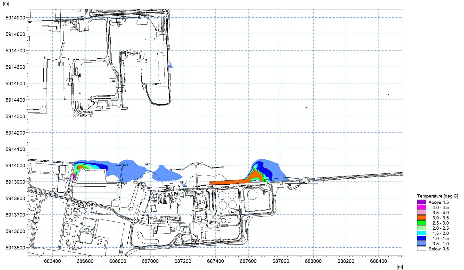
Figure 1.121: Thermal plume 9<sup>th</sup> April 2019 – excess temperature at high water circa 1.8m depth layer 3
