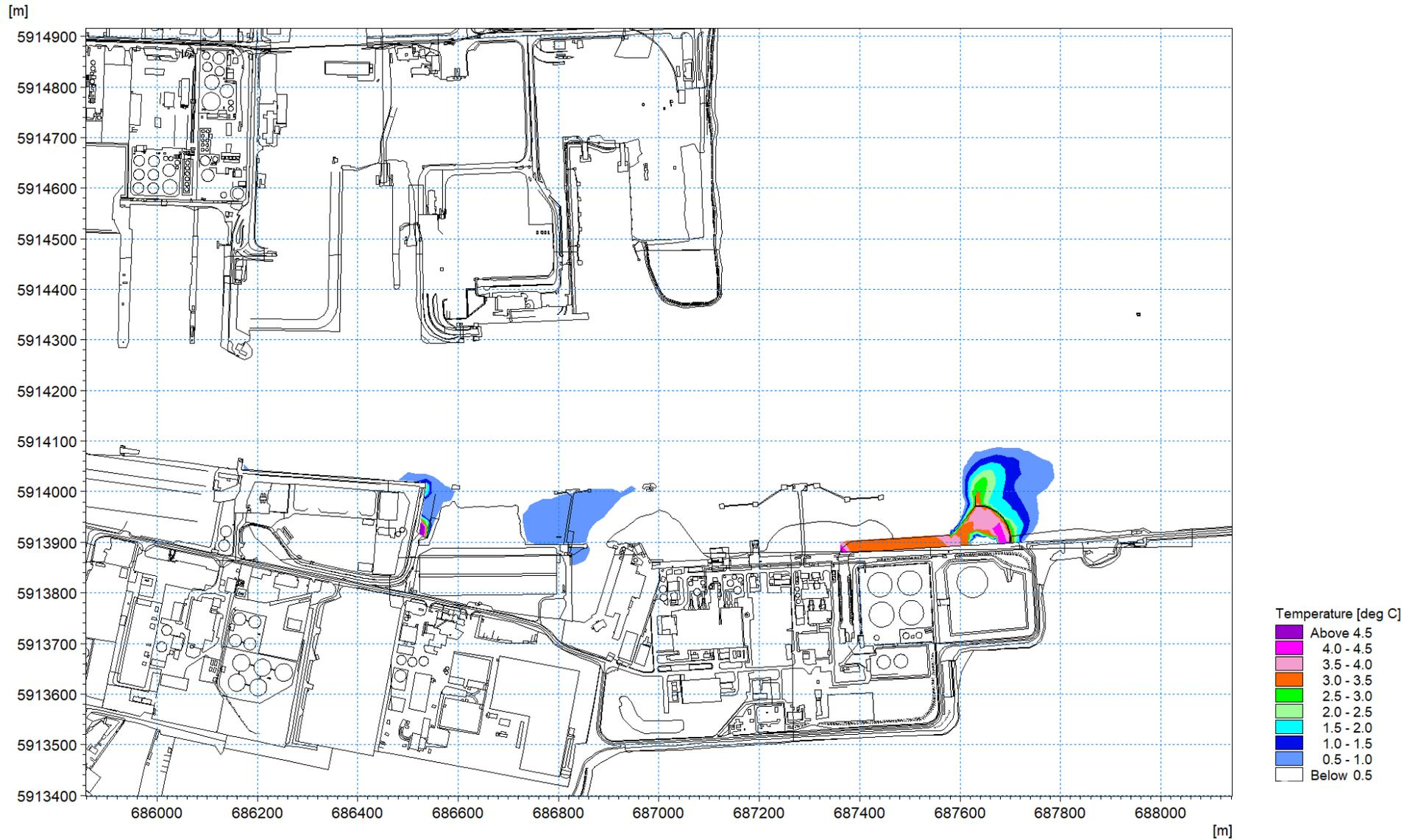
Figure 1.118: Thermal plume 9<sup>th</sup> April 2019 – excess temperature at mid-flood circa 1.8m depth layer 4
