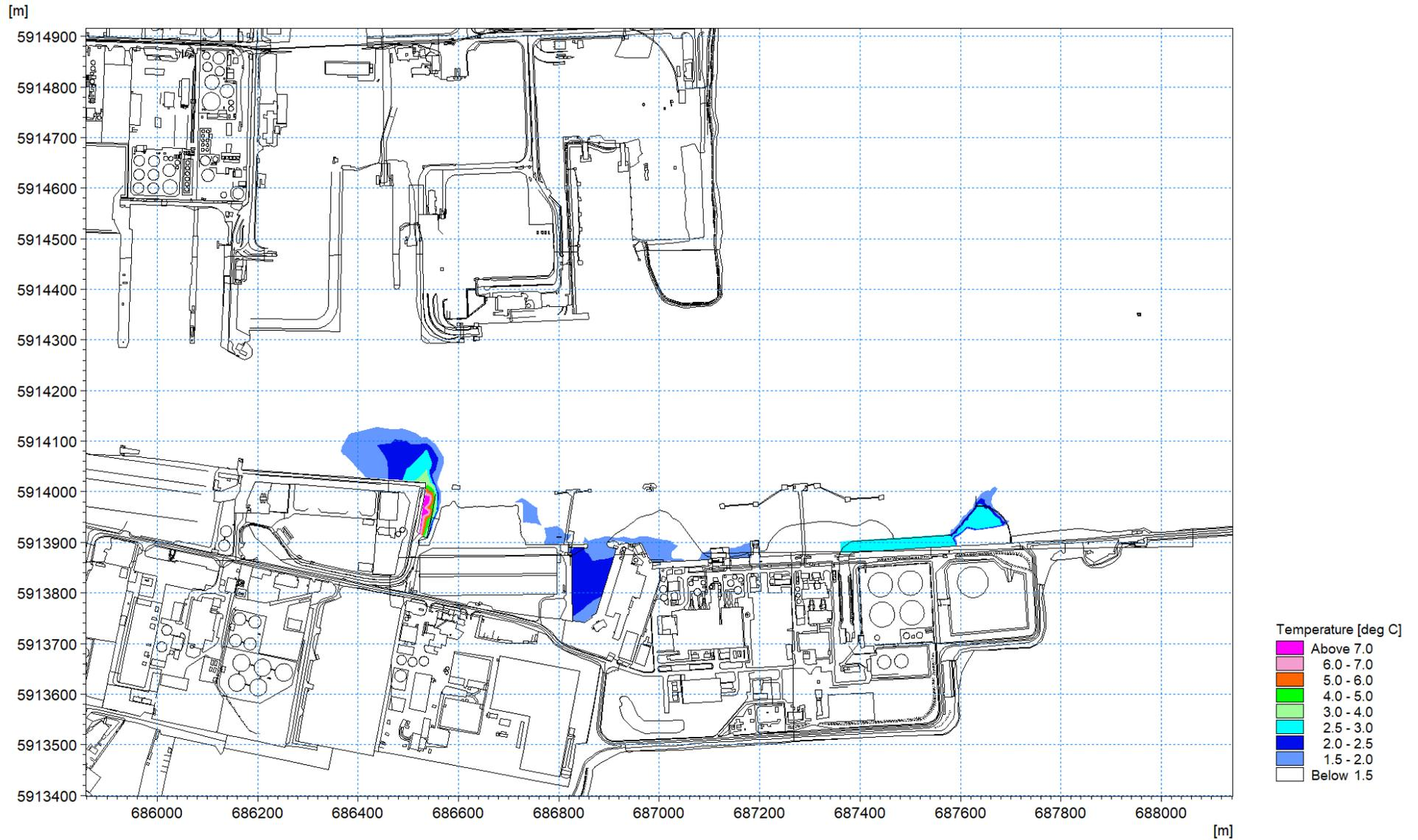
Figure 1.84: Thermal plume 20<sup>th</sup> April 2018 – excess temperature at mid-flood circa 2m depth layer 4
