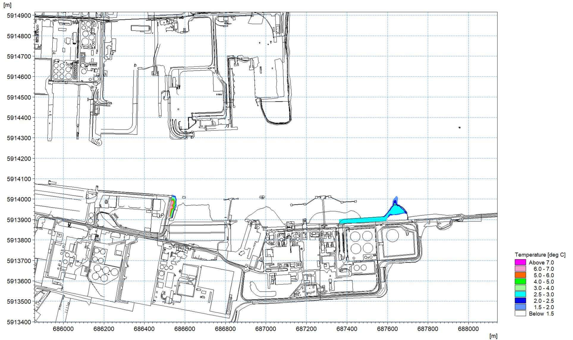
Figure 1.102: Thermal plume 24<sup>th</sup> April 2018 – excess temperature at mid-ebb circa 2m depth layer 4
