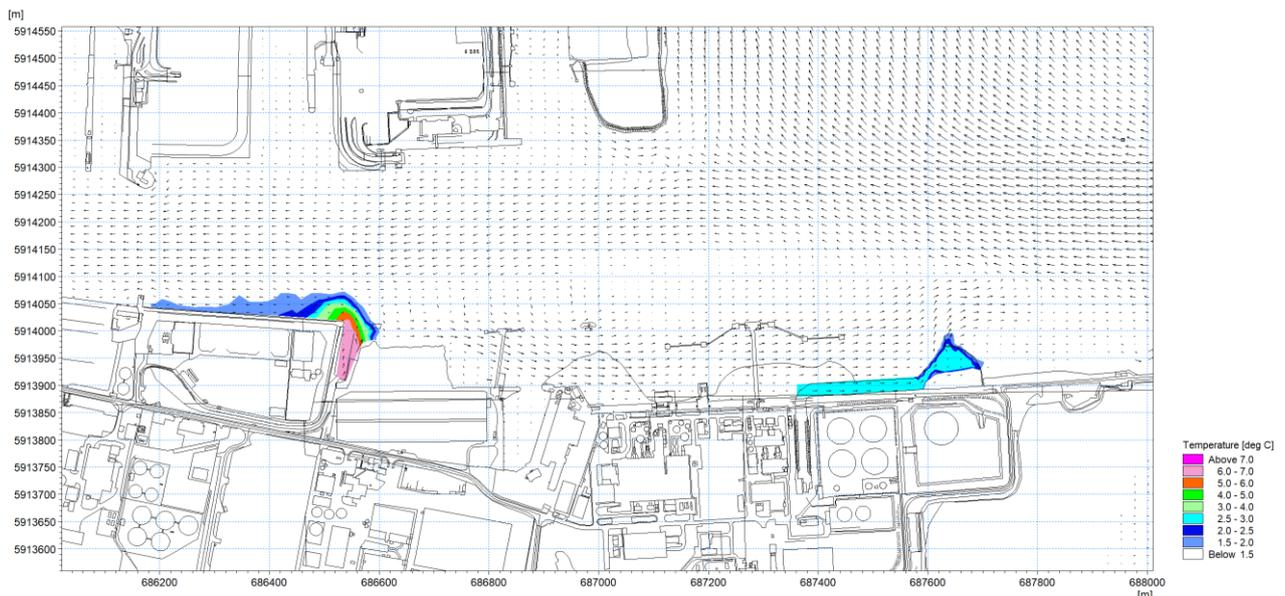
Figure 1.40: Thermal plume 20<sup>th</sup> April 2018 – excess temperature at low water circa 2m depth.
