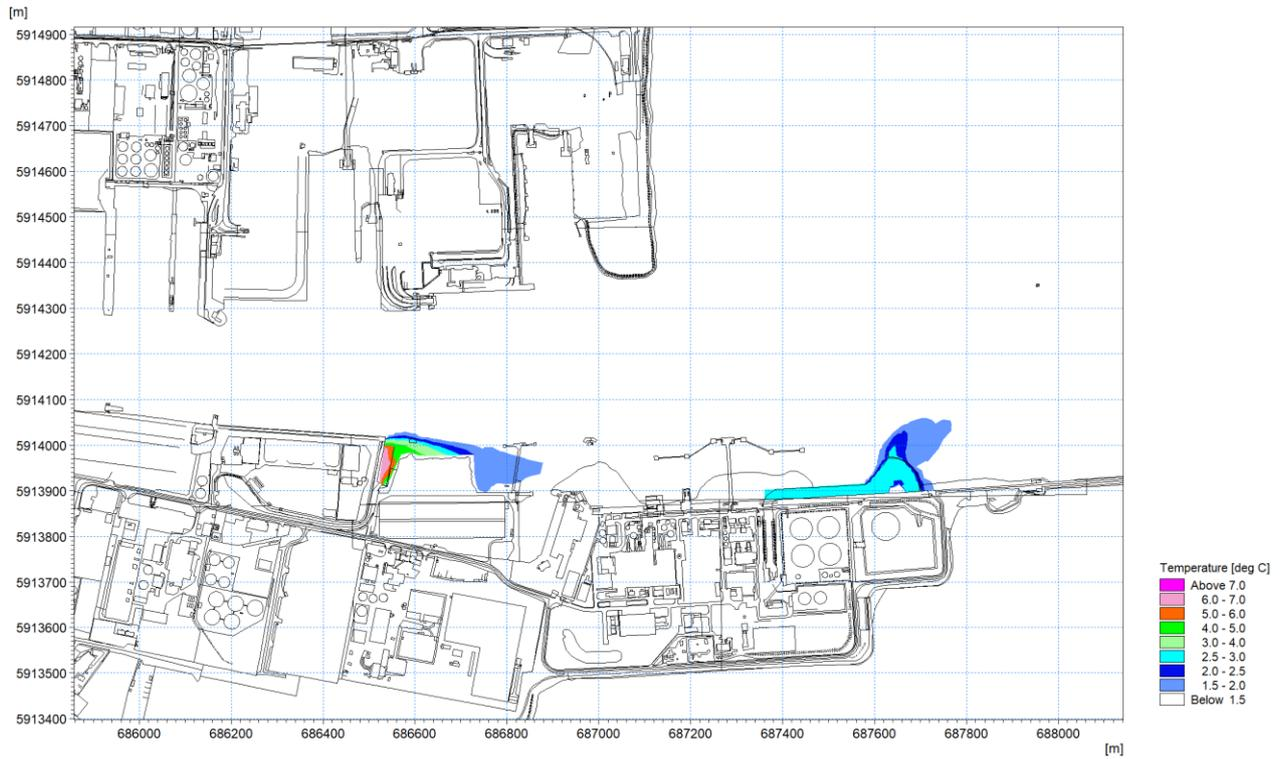
Figure 1.23: Thermal plume 20<sup>th</sup> April 2018 – excess temperature at high water circa 0.3m depth.
