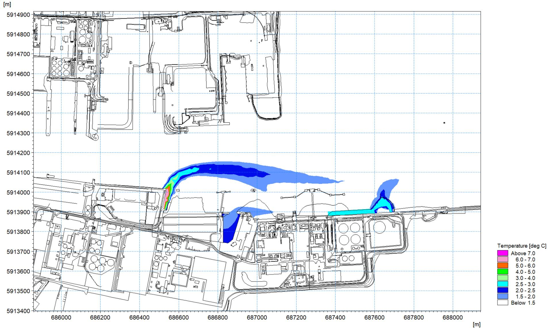
Figure 1.106: Thermal plume 24<sup>th</sup> April 2018 – excess temperature at mid-flood circa 0.3m depth layer 6
