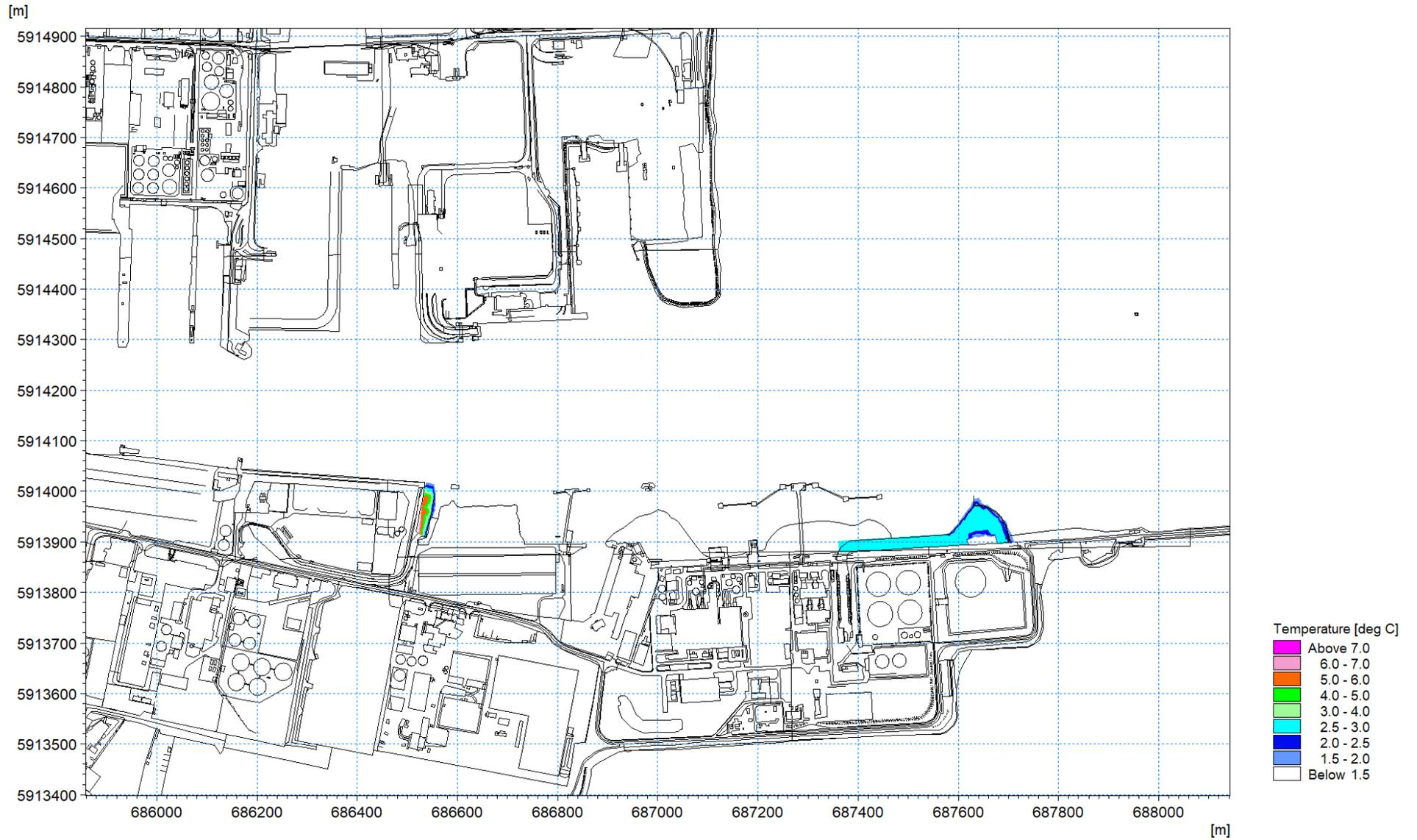
Figure 1.99: Thermal plume 24<sup>th</sup> April 2018 – excess temperature at high water circa 2m depth layer 4
