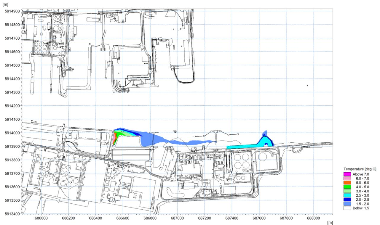
Figure 1.24: Thermal plume 20<sup>th</sup> April 2018 – excess temperature at high water circa 1m depth.
