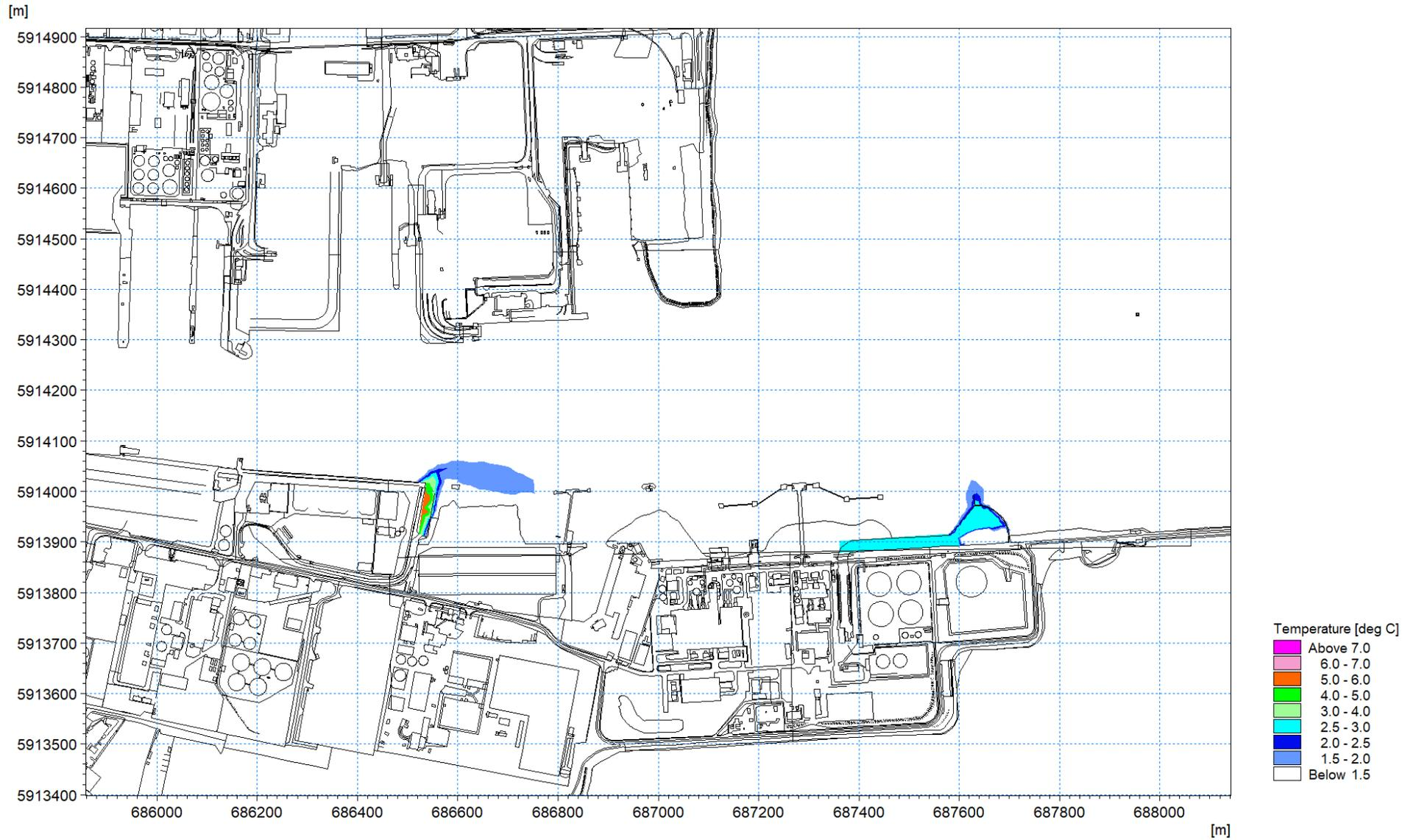
Figure 1.80: Thermal plume 12<sup>th</sup> August 2016 – excess temperature at mid-flood circa 1m depth layer 5
