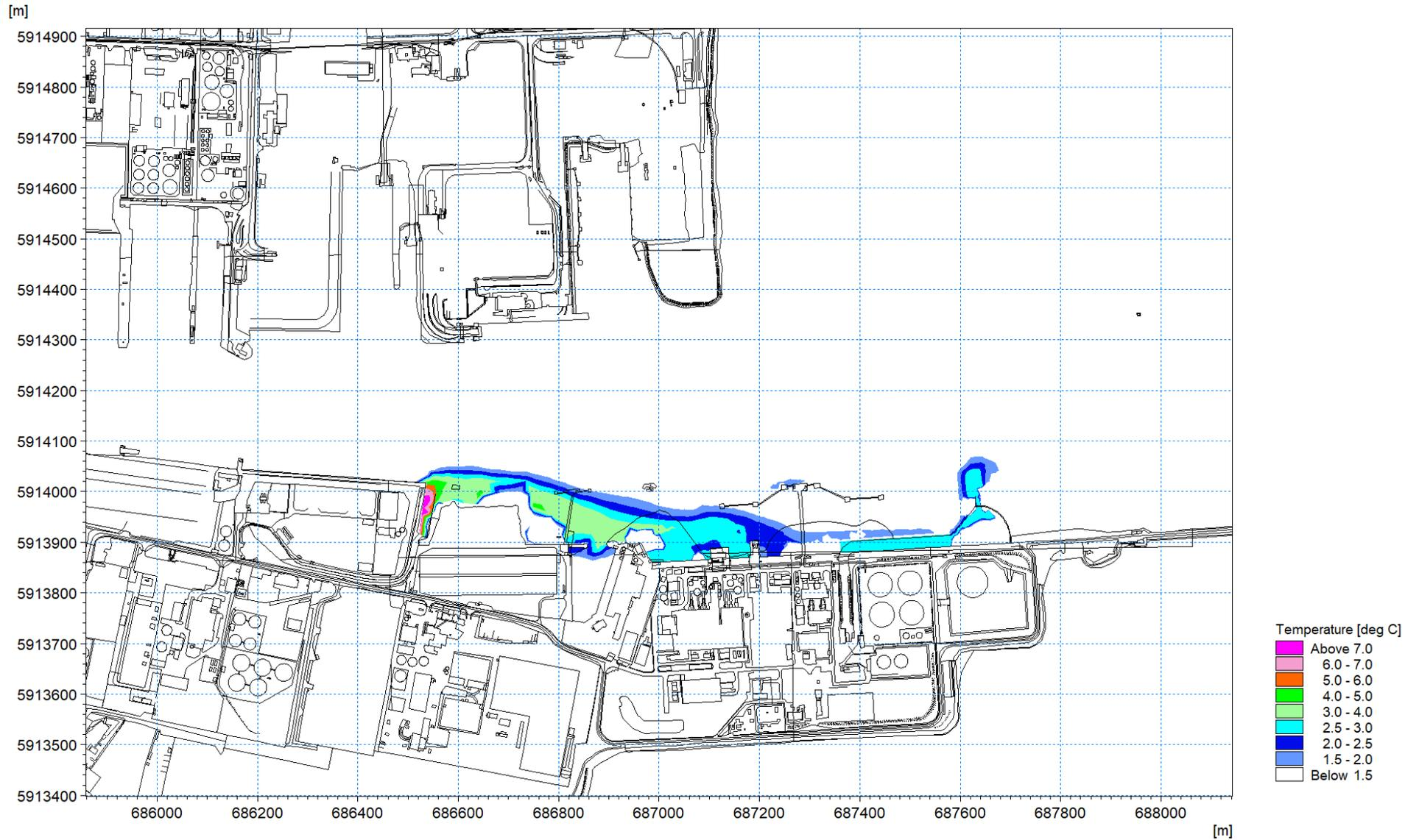
Figure 1.93: Thermal plume 20<sup>th</sup> April 2018 – excess temperature at low water circa 2m depth layer 4
