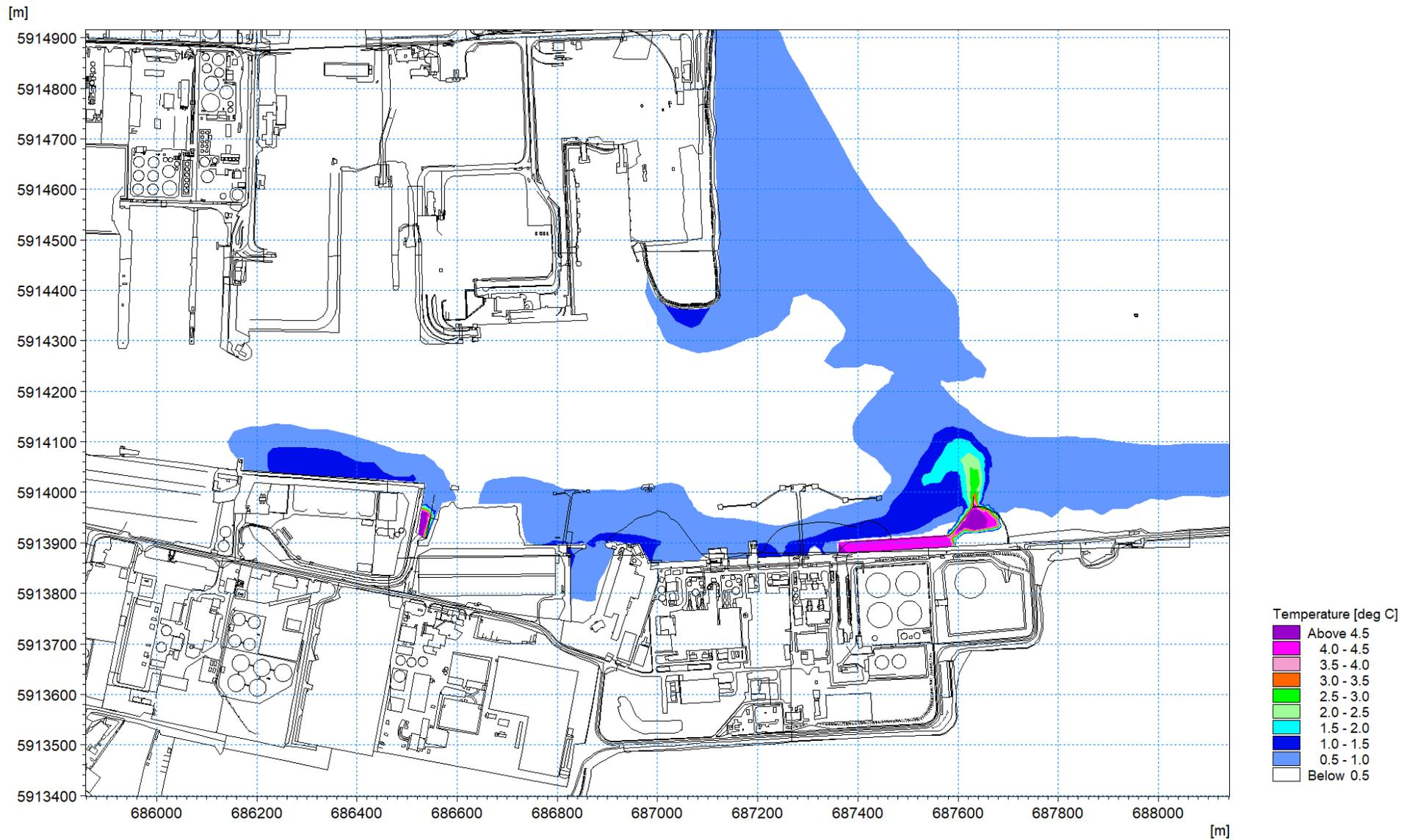
Figure 1.115: Thermal plume 9<sup>th</sup> April 2019 – excess temperature at low water circa 1.8m depth
