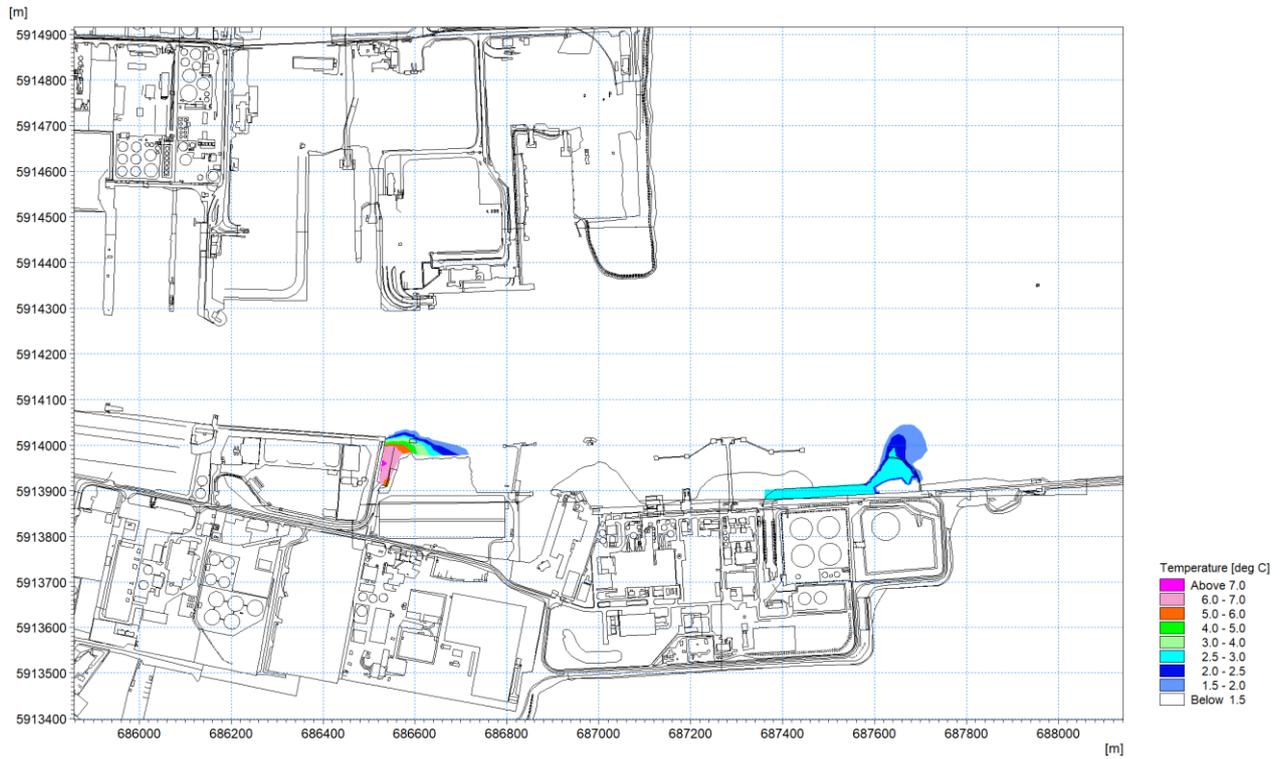
Figure 1.27: Thermal plume 20<sup>th</sup> April 2018 – excess temperature at mid-ebb circa 0.3m depth.
