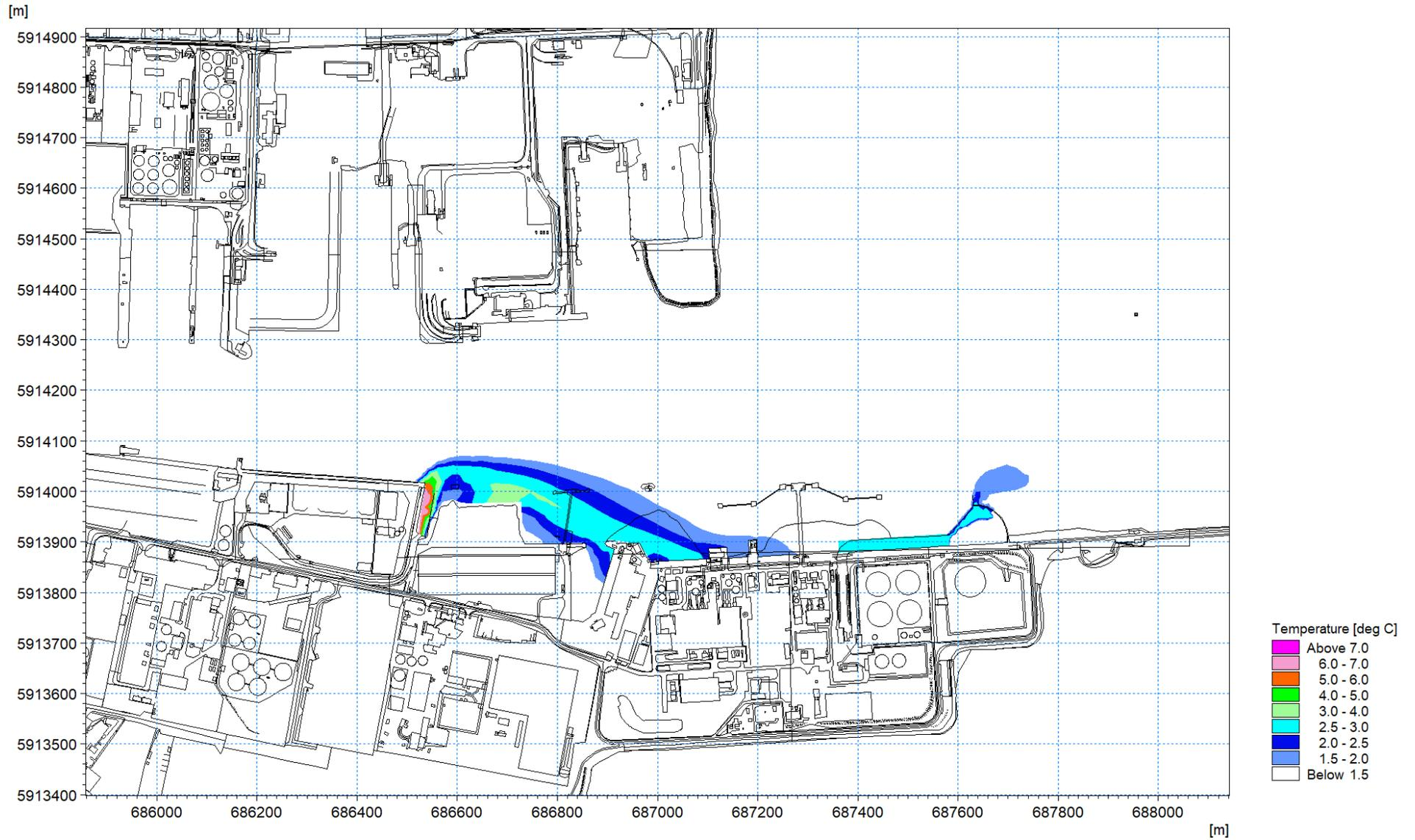
Figure 1.104: Thermal plume 24<sup>th</sup> April 2018 – excess temperature at low water circa 1m depth layer 5
