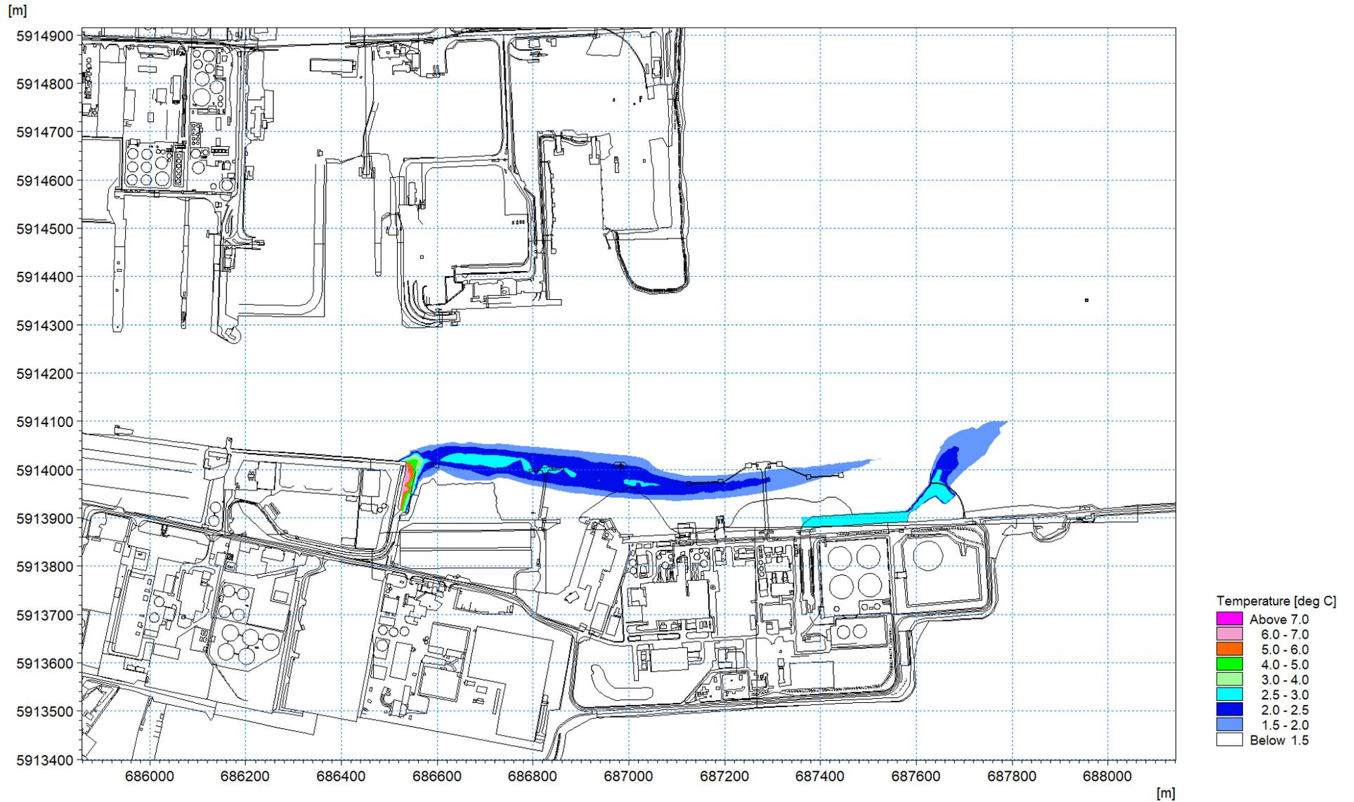
Figure 1.73: Thermal plume 12<sup>th</sup> August 2016 – excess temperature at mid-ebb circa 0.3m depth layer 6
