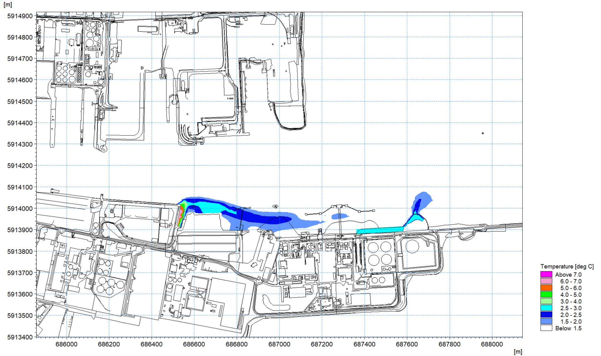
Figure 1.77: Thermal plume 12<sup>th</sup> August 2016 – excess temperature at low water circa 1m depth layer 5
