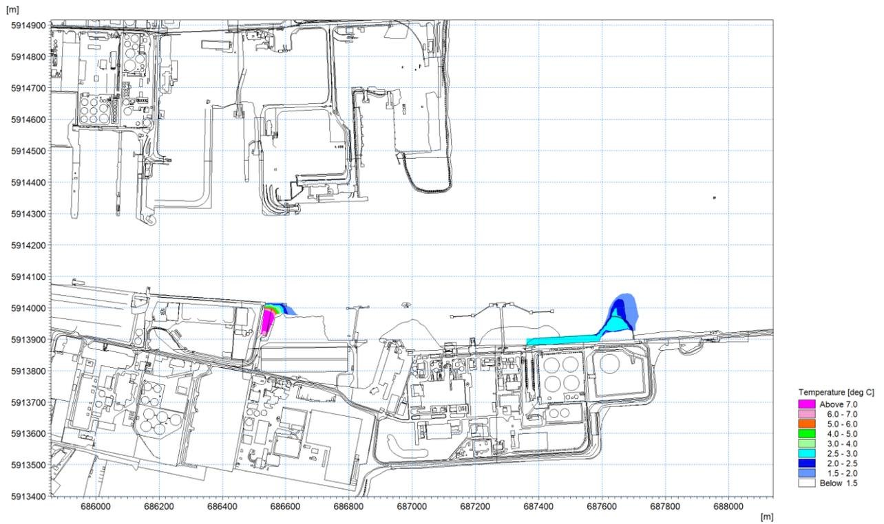
Figure 1.19: Thermal plume 20<sup>th</sup> April 2018 – excess temperature at mid-flood circa 0.3m depth.
