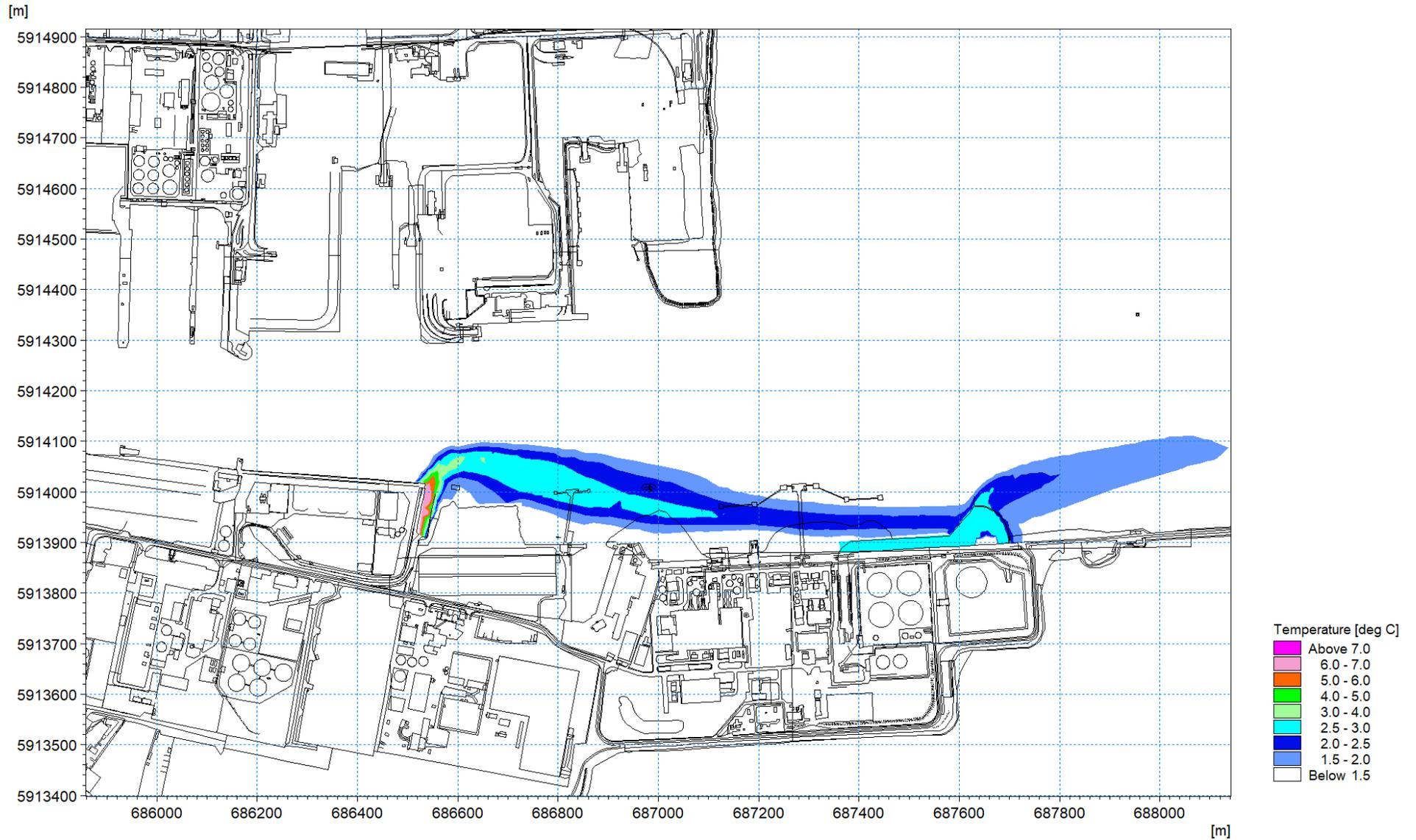
Figure 1.85: Thermal plume 20<sup>th</sup> April 2018 – excess temperature at high water circa 0.3m depth layer 6
