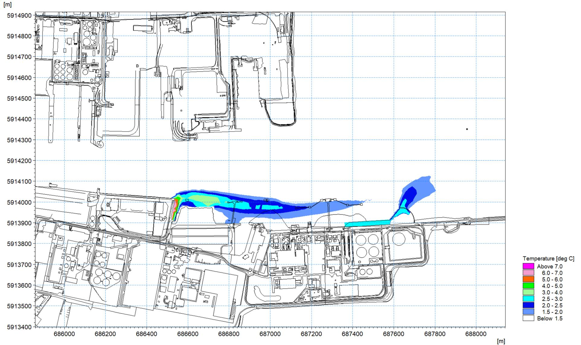
Figure 1.76: Thermal plume 12<sup>th</sup> August 2016 – excess temperature at low water circa 0.3m depth layer 6
