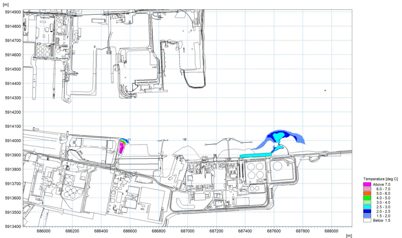
Figure 1.32: Thermal plume 20<sup>th</sup> April 2018 – excess temperature at low water circa 1m depth.
