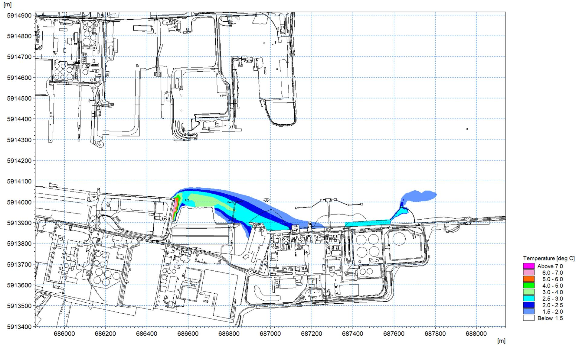
Figure 1.103: Thermal plume 24<sup>th</sup> April 2018 – excess temperature at low water circa 0.3m depth layer 6
