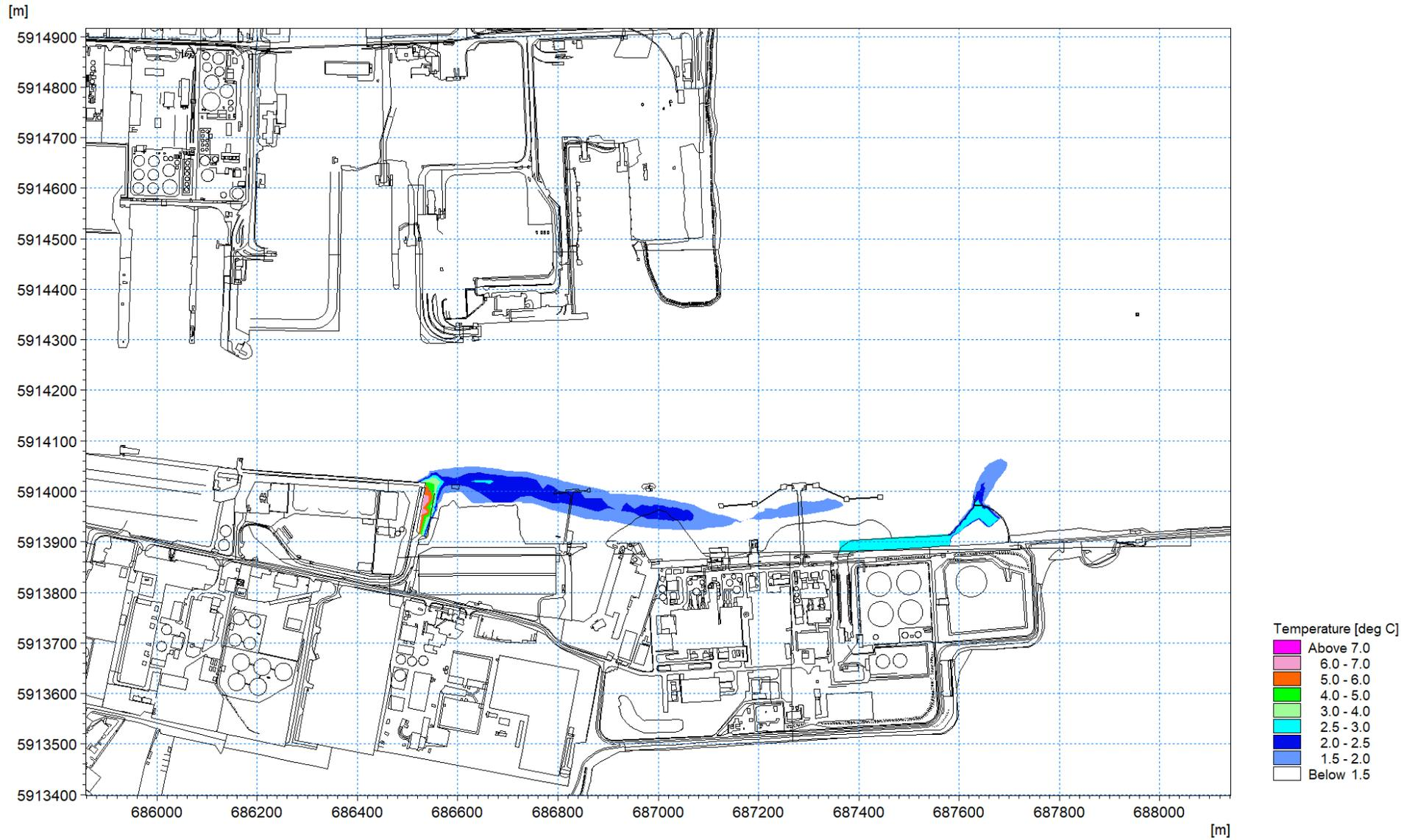
Figure 1.74: Thermal plume 12<sup>th</sup> August 2016 – excess temperature at mid-ebb circa 1m depth layer 5
