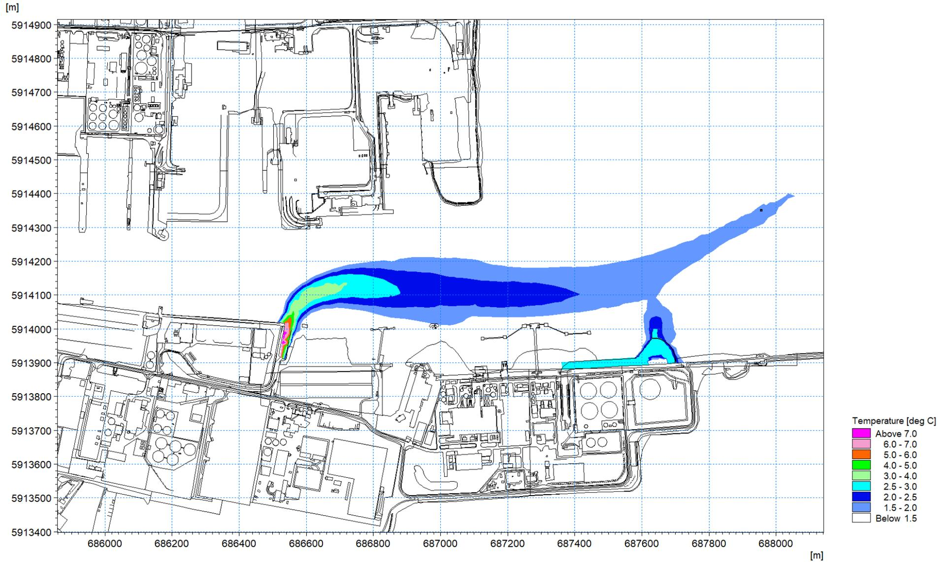
Figure 1.97: Thermal plume 24<sup>th</sup> April 2018 – excess temperature at high water circa 0.3m depth layer 6
