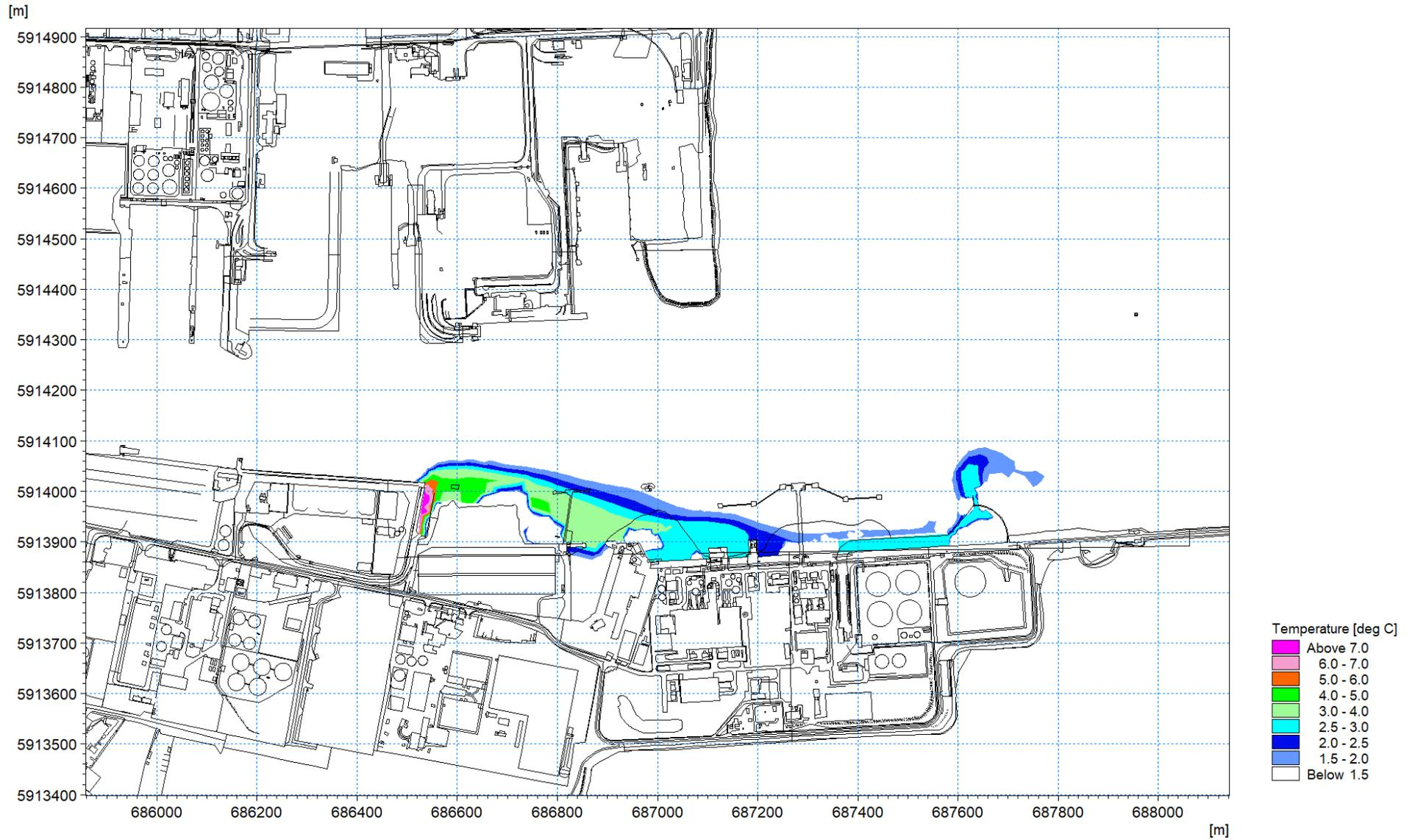
Figure 1.92: Thermal plume 20<sup>th</sup> April 2018 – excess temperature at low water circa 1m depth layer 5
