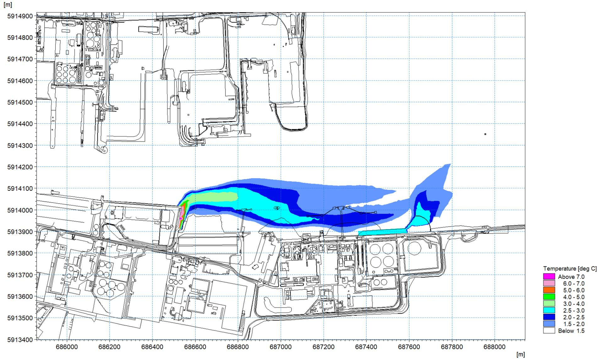
Figure 1.88: Thermal plume 20<sup>th</sup> April 2018 – excess temperature at mid-ebb circa 0.3m depth layer 6
