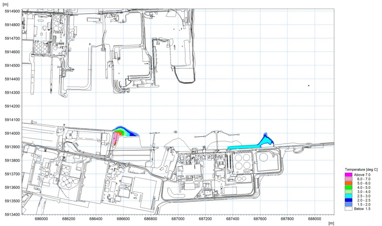
Figure 1.28: Thermal plume 20<sup>th</sup> April 2018 – excess temperature at mid-ebb circa 1m depth.
