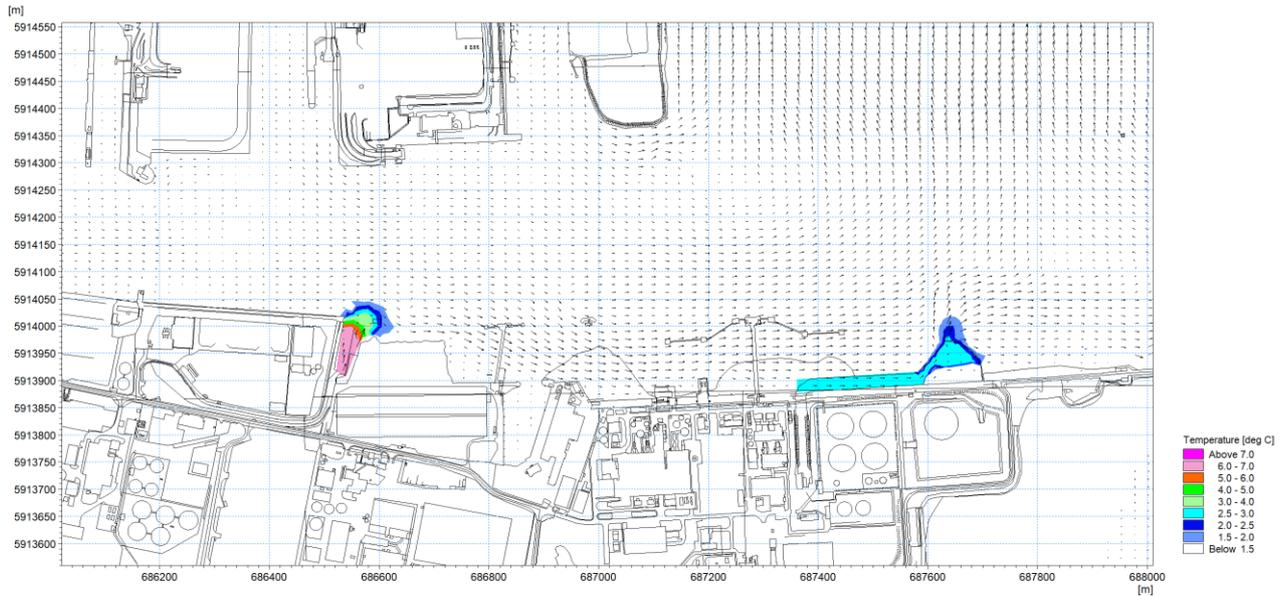
Figure 1.39: Thermal plume 24<sup>th</sup> April 2018 – excess temperature at mid-flood circa 1m depth.
