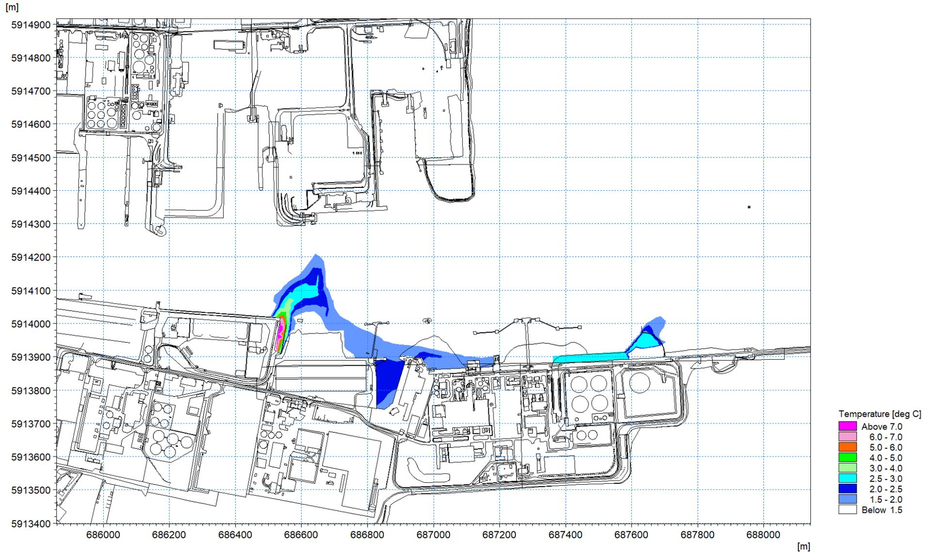
Figure 1.83: Thermal plume 20<sup>th</sup> April 2018 – excess temperature at mid-flood circa 1m depth layer 5
