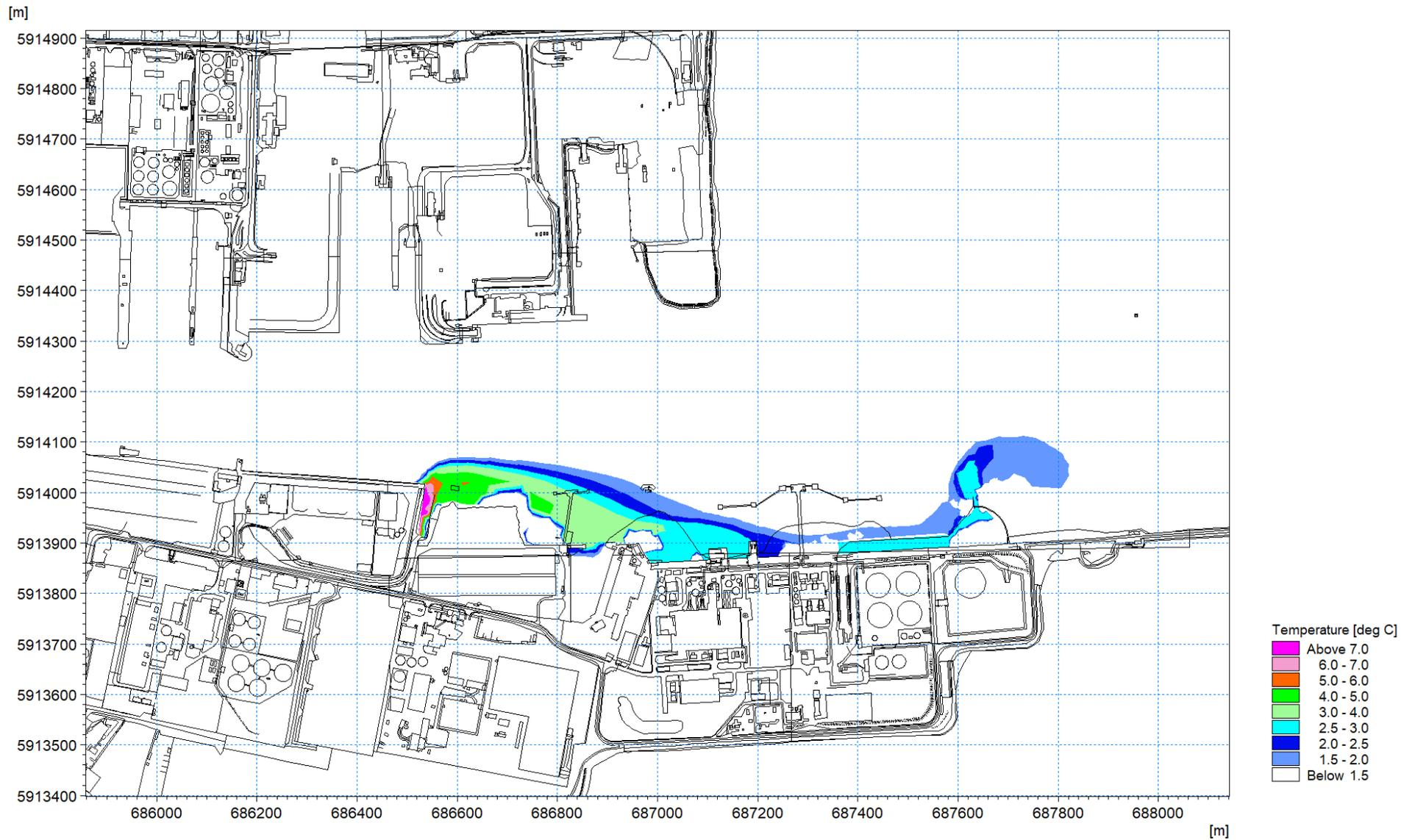
Figure 1.91: Thermal plume 20<sup>th</sup> April 2018 – excess temperature at low water circa 0.3m depth layer 6
