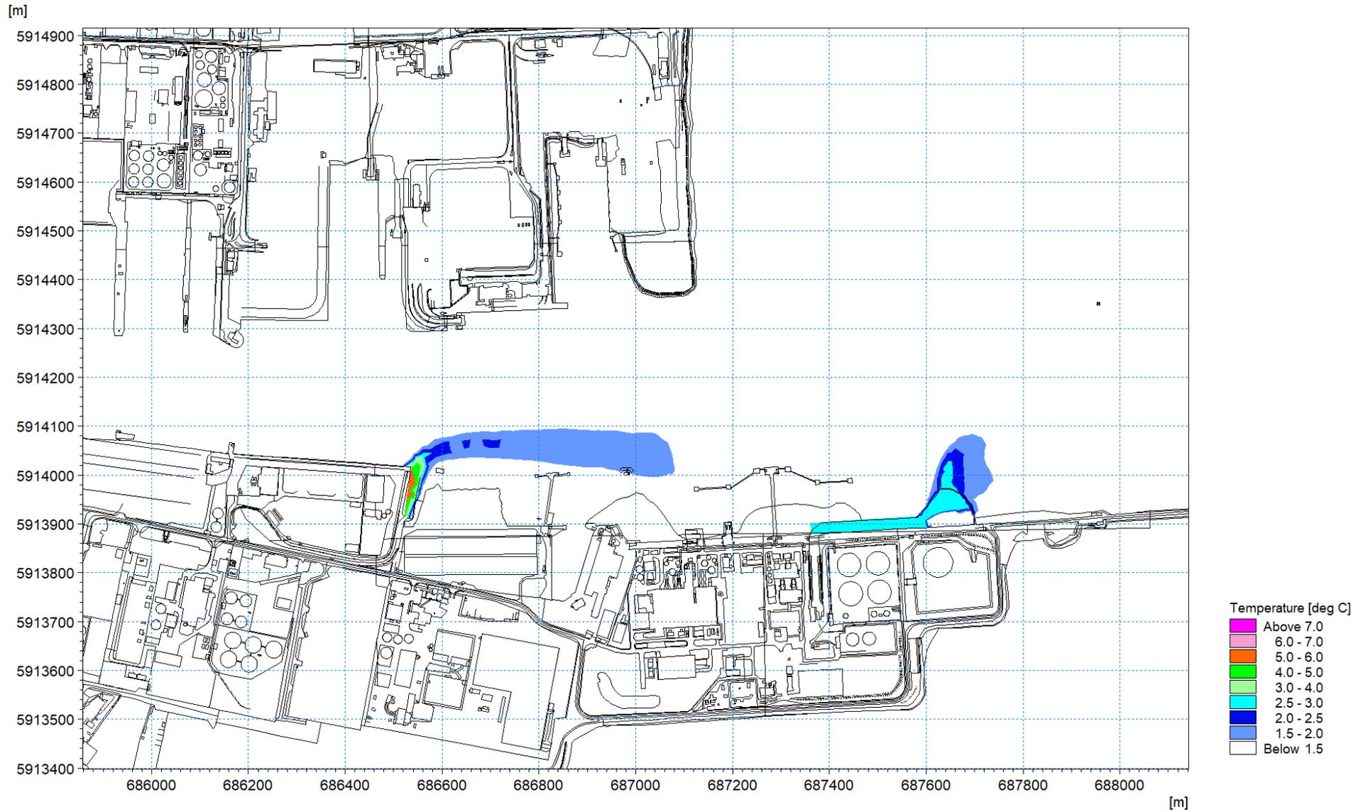
Figure 1.70: Thermal plume 12<sup>th</sup> August 2016 – excess temperature at high water circa 0.3m depth layer 6
