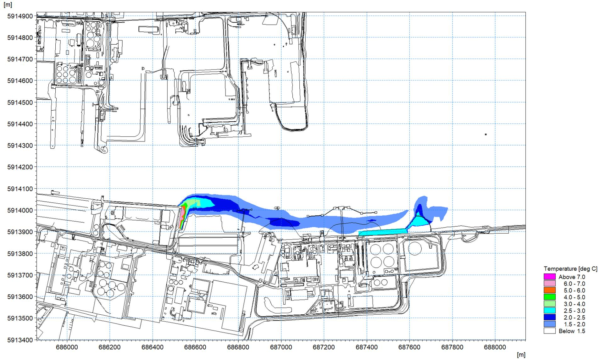
Figure 1.89: Thermal plume 20<sup>th</sup> April 2018 – excess temperature at mid-ebb circa 1m depth layer 5
