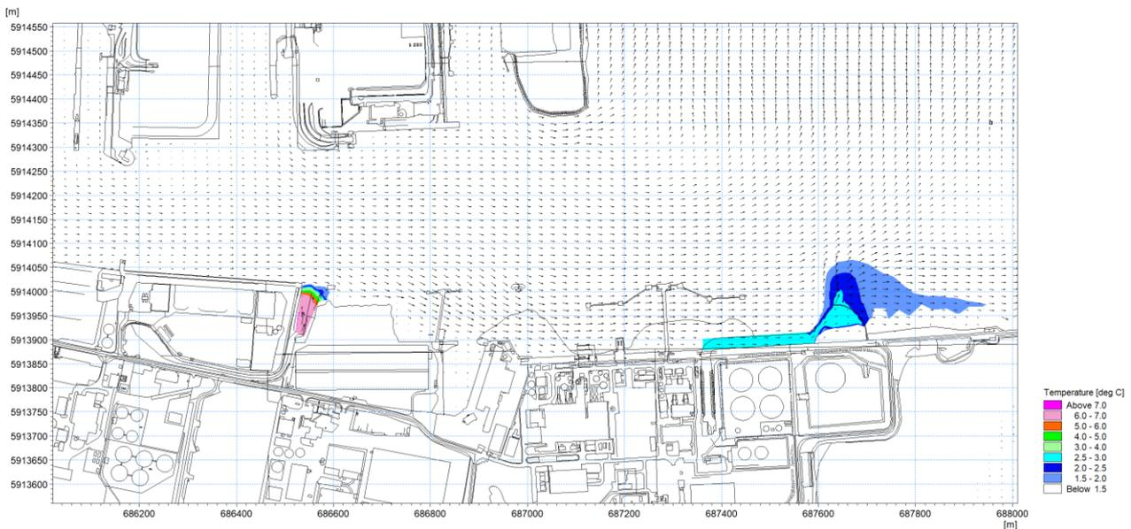
Figure 1.38: Thermal plume 24<sup>th</sup> April 2018 – excess temperature at mid-flood circa 0.3m depth.
